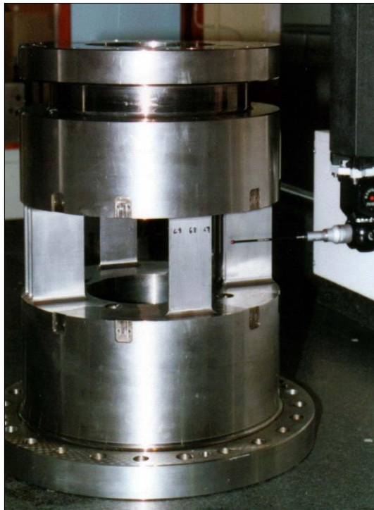
Bare balance structure being inspected just prior to the gauge installation
