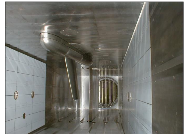
Commissioning Half Model (CHM) in the ETW test section
